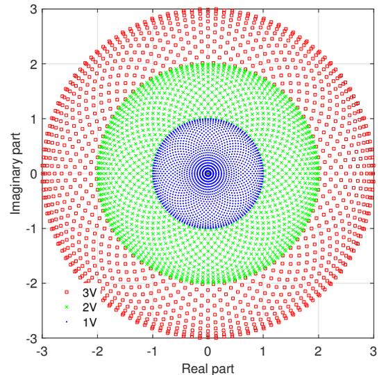
Fig. 6. Ideal constellation diagram for DPWPM combined with a 4-level SMPA.
