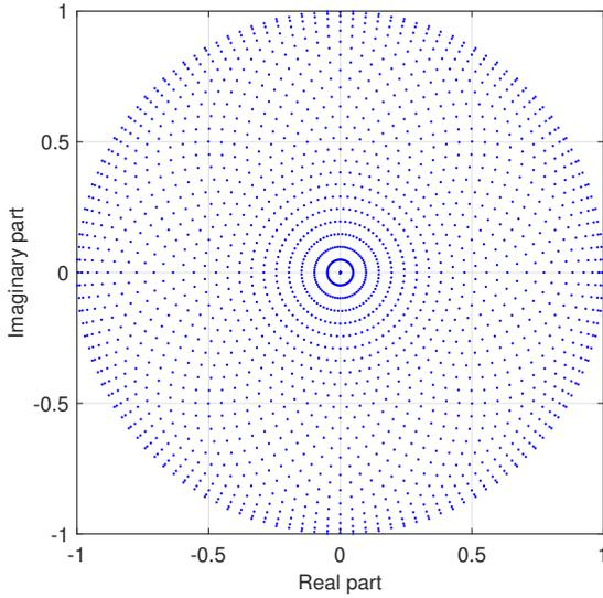
Fig. 3. Ideal constellation diagram for a DPWPM with a 2-level SMPA.
