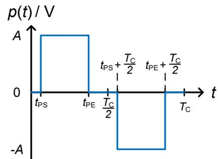
Fig. 2. Bipolar output pulse of an ideal DPWPM.
