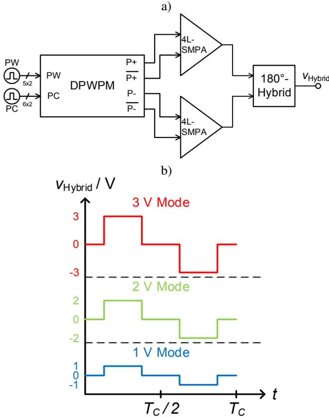
Fig. 5. a) Block diagram of the proposed DPWPM-4L-SMPA-system. b) Output signal with possible output swings of the 4L-SMPA.
