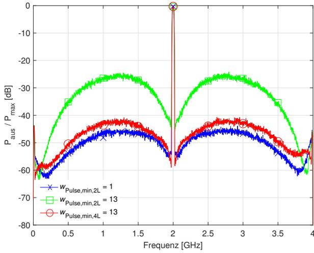
Fig. 7. Simulated normalized output spectra of the ideal DPWPM with a 2L-SMPA using the conventional constellation diagram (Fig.3) and a 4L-SMPA using the enhanced constellation diagram (Fig. 6).
