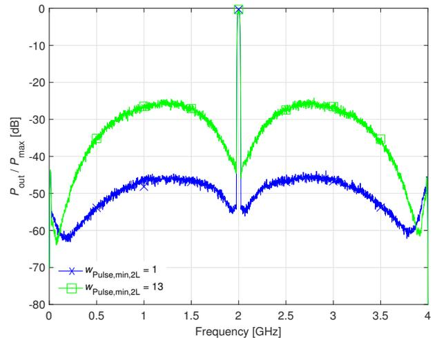
Fig. 4. Simulated normalized output spectra of the ideal DPWPM with a conventional two-level (2L) constellation diagram depicted in Fig. 3 and the pulse-width limit  $w_{\text{Pulse,min,2L}}$  set to 1 (ideal case) and 13 (realistic case).
