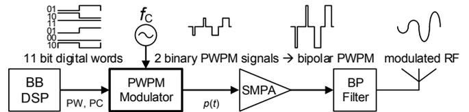
Fig. 1. RF transmitter chain with bipolar DPWPM modulator, SMPA and bandpass reconstruction filter [1].
