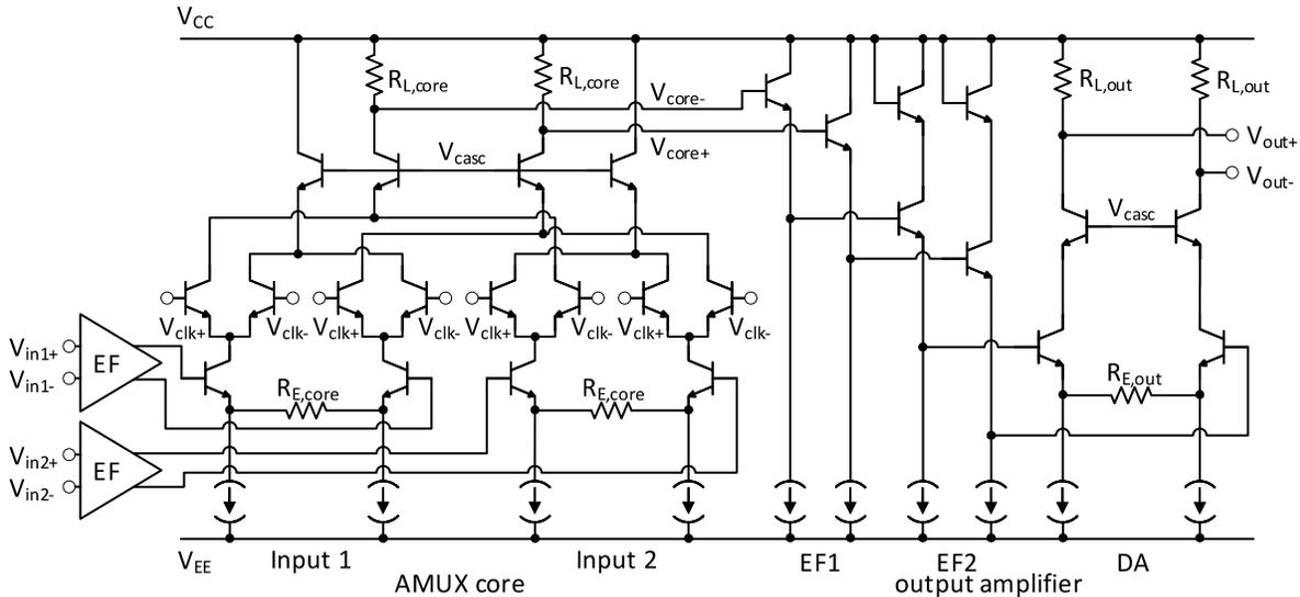
Fig. 3. Schematic of AMUX core and output amplifier.
