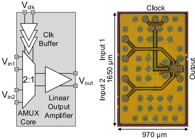
Fig. 2. AMUX block diagram and chip photograph.
