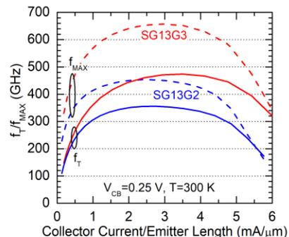
Fig. 1. Measured  $f_T$  and  $f_{MAX}$  as a function of collector current per emitter length for both technologies. Devices with eight emitters of 1  $\mu\text{m}$  length in parallel were measured. The emitter width is 130 nm for the SG13G2 device and 110 nm for the SG13G3 device.
