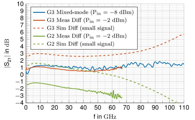
Fig. 6. Differential and calculated mixed-mode signal path transmission  $S_{21}$ . Two measurements for SG13G3 chip compared to SG13G2 and small signal simulation. Input power indication is single-ended.
