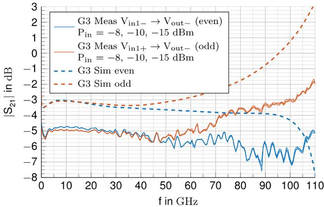
Fig. 5. Single-ended signal path transmission  $S_{21}$ . Measurement for different input powers and small signal simulation of SG13G3 chip. Pin configurations “even” and “odd”.
