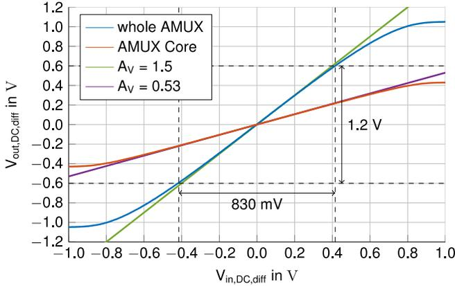
Fig. 4. Simulated static transfer characteristic of the AMUX. Curves for AMUX core without output amplifier and whole AMUX with output amplifier. The linear nominal operating region is indicated by dashed lines.
