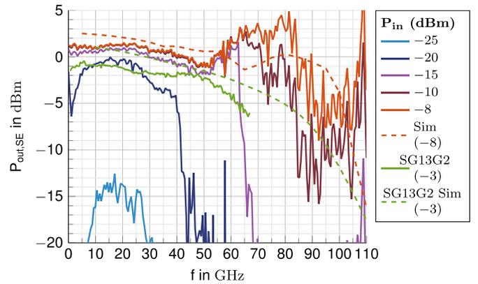
Fig. 8. Single-ended clock path output power for different input powers. Compared to differentially measured SG13G2 chip and large signal simulation. All input and output power indications are single-ended.
