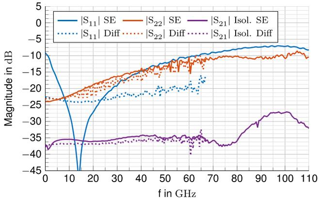
Fig. 7. Measured reflection coefficients  $S_{11}$  and  $S_{22}$  and transmission  $S_{21}$  for the inactive signal path of SG13G3 chip.
