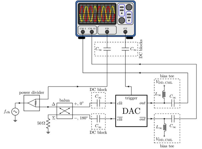
Fig. 15. Measurement setup (PR: phase reference, PT: prescale trigger).
