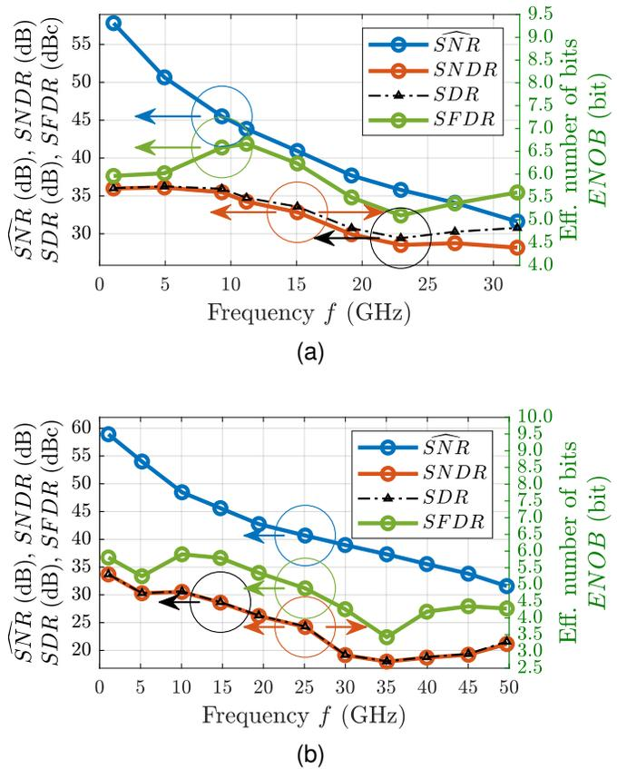
Fig. 17. Dynamic characterization results at (a) 64 GS/s and (b) 100 GS/s.
