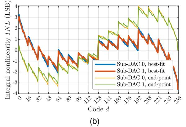
Fig. 16. Results of the static characterization measured at 50-GS/s sub-DAC operation corresponding to 100-GS/s operation with activated AMUX. (a)  $DNL$  and (b)  $INL$ .
