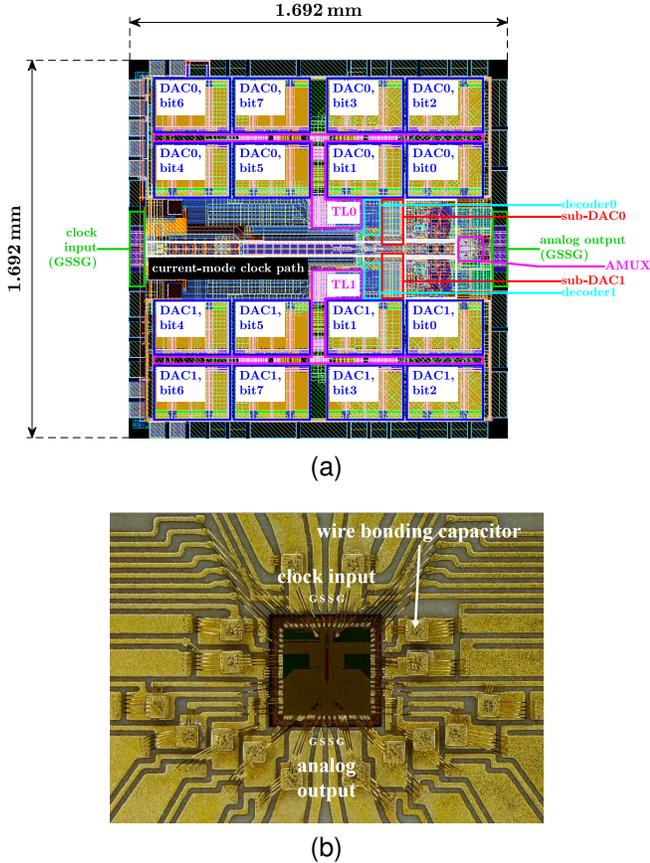
Fig. 13. (a) Layout of the chip with different circuit parts being highlighted and (b) micrograph of the bonded die in RF PCB cavity. Transmission lines TL0/1 denote the data paths from the memory to the sub-DAC cores.
