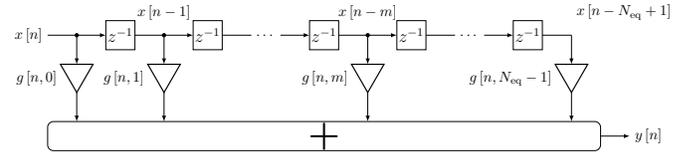
Fig. 14. Discrete-time, time-varying finite impulse response filter applied for LPTV predistortion with an input signal  $x[n]$  and output signal  $y[n]$  [49].
