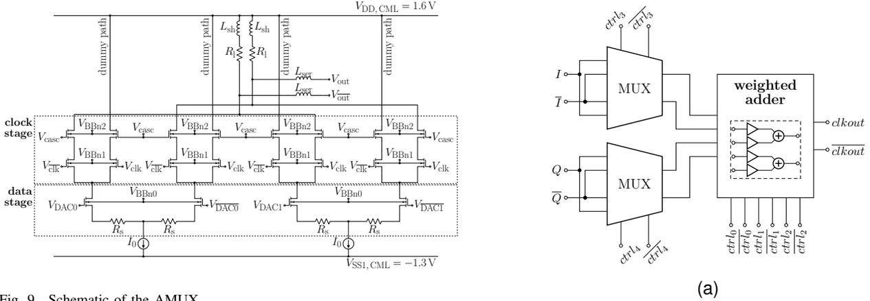
Fig. 9. Schematic of the AMUX.
