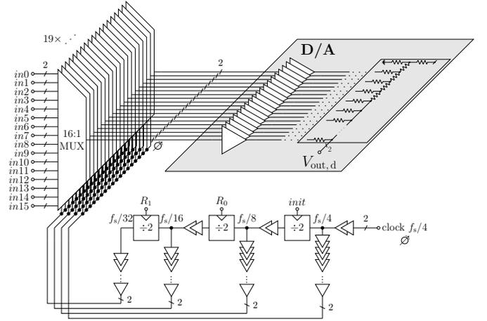
Fig. 5. Block diagram of one sub-DAC core. Common-mode voltages can be measured at the positions marked by  $\phi$ .
