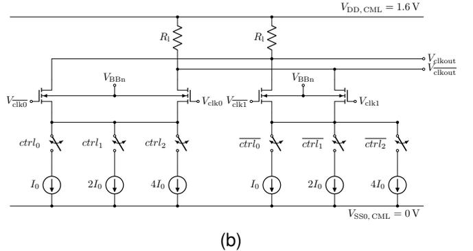
Fig. 10. Implementation of the quadrature phase rotators. (a) MUX stage selecting the quadrant and (b) phase interpolator.
