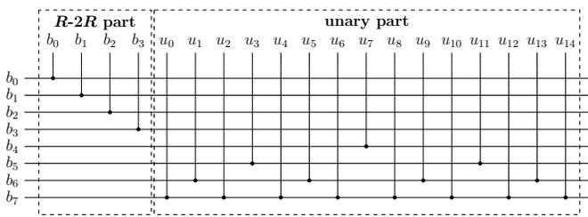
Fig. 4. Passive decoding network for the pseudo-segmented architecture [28], [29]. It shows the mapping of the 8 bits  $b_0, \dots, b_7$  to the 19 DAC channels:  $R$ - $2R$  part  $b_0, \dots, b_3$  and unary part  $u_0, \dots, u_{14}$ .
