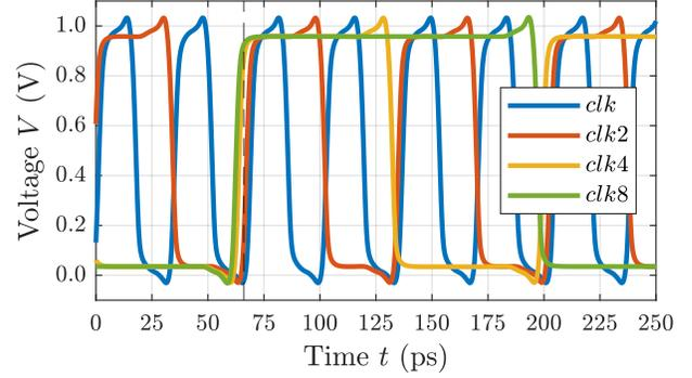
Fig. 12. Simulation of clock signals on schematic level at the output of the clock network in Fig. 5 (single-ended) at  $f_s = 118$  GS/s. Clock signals correspond to the MUX tree clock inputs in Fig. 7a.
