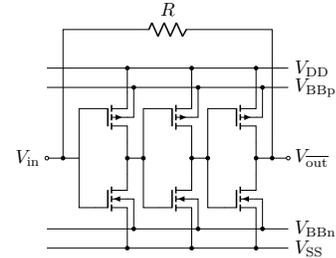
Fig. 6. Resistive feedback concept in the clock driver chains of the sub-DACs.  $V_{BBn}$  and  $V_{BBp}$  represent the body-biasing voltages for forward body-biasing.
