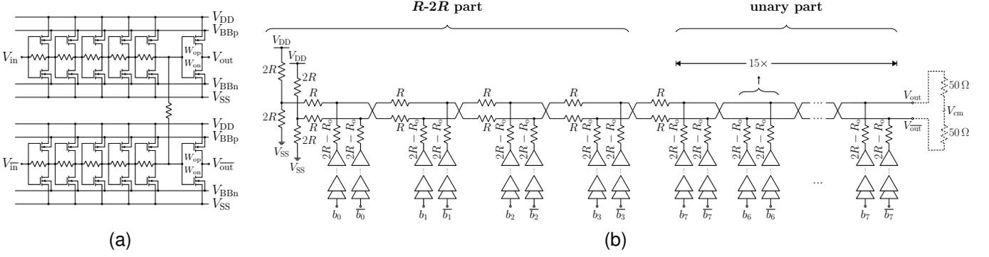
Fig. 8. (a) Output driver stage in the sub-DACs and (b) schematic of the output network realizing the digital-to-analog conversion with driver stages according to (a) and a resistor network. Unary paths are connected in an alternating arrangement  $b_7$ - $b_6$ - $b_7$ - $b_5$ - $b_7$ - $b_6$ - $b_7$ - $b_4$ - $b_7$ - $b_6$ - $b_7$ - $b_5$ - $b_7$ - $b_6$ - $b_7$ .
