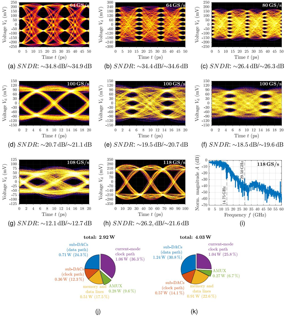
Fig. 20. Measured PAM eye diagrams (differential signals). (a) 64 GS/s PAM-4, (b) 64 GS/s PAM-8, (c) 80 GS/s PAM-8, (d) 100 GS/s PAM-2, (e) 100 GS/s PAM-4, (f) 100 GS/s QPRBS-13, (g) 108 GS/s PAM-2 and (h) 118 GS/s PAM-2 with oversampling and raised-cosine pulse shaping (roll-off factor  $\beta = 0.5$ ). In (i), the spectrum of the signal in (h) is shown. Power breakdowns at 64 GS/s and 100 GS/s are depicted in (j) and (k), respectively. Finally,  $SNDR$  values are given for both eye openings.
