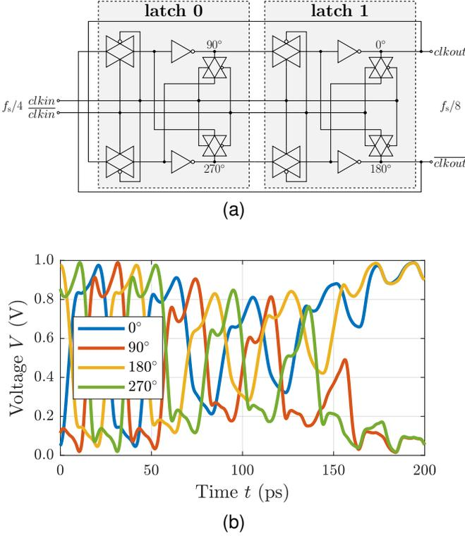
Fig. 11. (a) Implementation of the first CMOS frequency divider. Initialization transistors are not shown. (b) Simulated behavior on schematic level at an input frequency of 48 GHz in case of a critical distortion (here: supply voltage drop).
