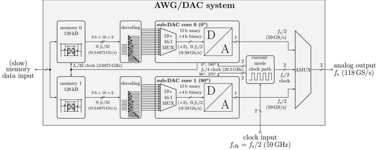
Fig. 2. AWG/DAC system overview. Two memory blocks with 128 kB each provide the data for the two sub-DAC cores with a nominal resolution of 8 bit. The analog outputs of the sub-DACs are combined by an active AMUX. Values in brackets are given for 118-GS/s operation.
