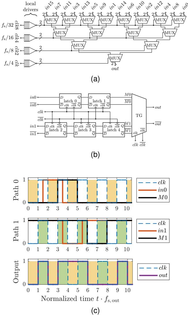
Fig. 7. (a) MUX tree resulting in a 16:1 serializer and (b) single MUX stage [34] with (c) corresponding timing diagram. Input inverters at each MUX stage are not drawn. For  $clk = H$ , latches are in opaque mode and for  $clk = L$ , they are transparent. Local drivers at each MUX tree reduce the load of the global clock network. The frequency  $f_{s,out}$  corresponds to the output data rate at the output of each MUX stage.
