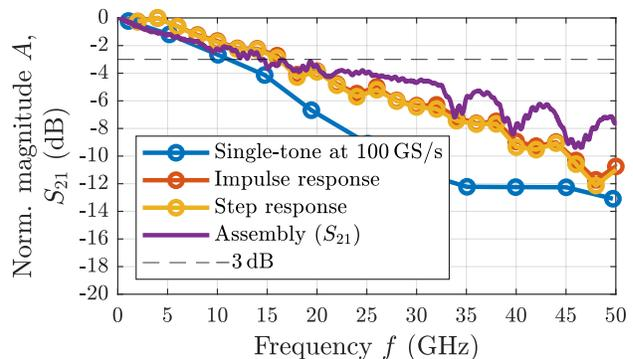
Fig. 19. Bandwidth estimation based on measurements at  $f_s = 100$  GS/s. The  $\sin(x)/x$  roll-off is compensated.
