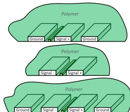
Figure 1: Overview of possible electrode topologies in simplified MZMs
