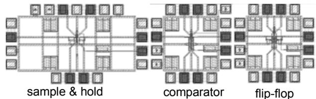
Figure 14. Layout of the ADC building blocks. Pad pitch 100  $\mu\text{m}$ .
