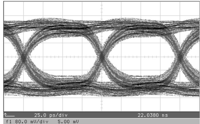
Figure 9. Measured sample & hold circuit output eye diagram with a 40 Gbit/s PRBS  $2^7-1$  input data stream at  $f_{clock} = 10$  GHz.
