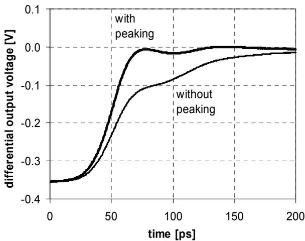
Figure 12. Measured comparator output voltage transient  $V_{out,D}(t)$  with peaking enabled ( $V_{peak} = V_{DD}$ ) and disabled ( $V_{peak} = V_{SS}$ ).  $V_{in,D}$  step from -500 mV to 0 mV at  $V_{comp,D} = 0$  mV.
