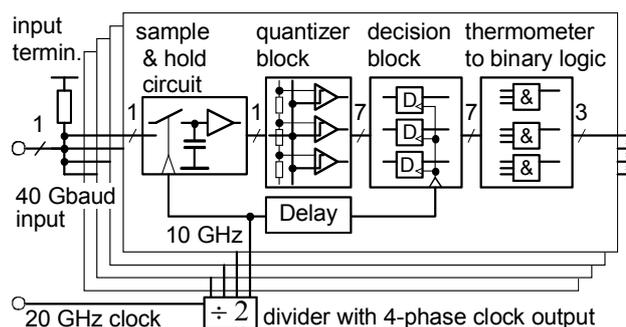
Figure 1. Concept of a 40-Gs/s ADC consisting of four time-interleaved 10-Gs/s flash ADCs.
