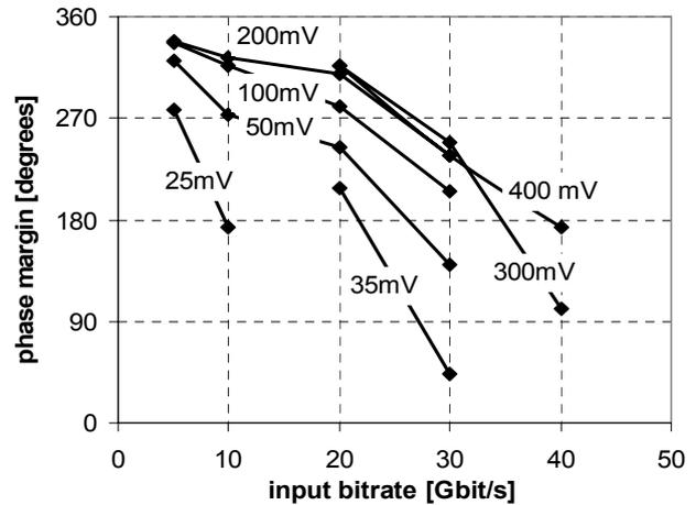
Figure 13. Phase margin of flip-flop versus input bit rate. Single-ended input voltage swing as parameter.
