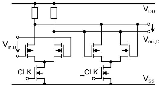
Figure 8. Schematic of the D-latch.
