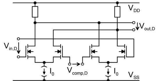
Figure 5. Schematic of the comparator input stage.
