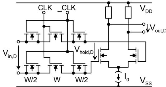
Figure 3. Schematic of the track & hold circuit.
