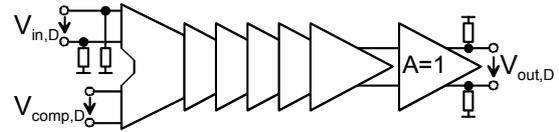
Figure 4. Block diagram of the comparator circuit.
