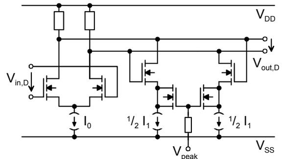
Figure 6. Schematic of the comparator gain stage with active peaking.
