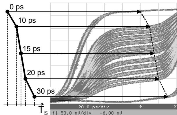
Figure 10. Reconstruction of the hold voltage  $V_{hold,D}(t)$  of the first track & hold stage in track mode by varying the sampling time  $T_s$ .
