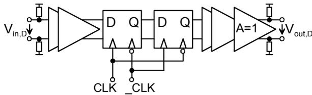
Figure 7. Block diagram of the flip-flop circuit.
