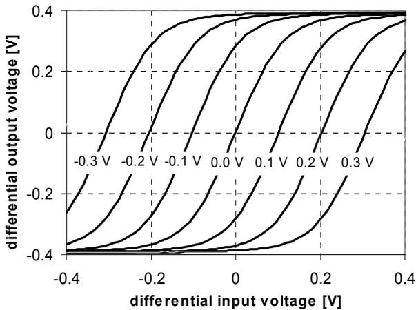
Figure 11. Measured comparator DC quantization characteristic with differential compare voltage  $V_{comp,D} = -0.3$  V to 0.3 V as parameter.
