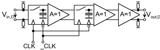
Figure 2. Block diagram of the sample & hold circuit.
